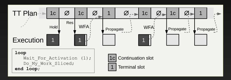
Work\_Control\_Block has all needed flags for the TT scheduler to handle propagation
